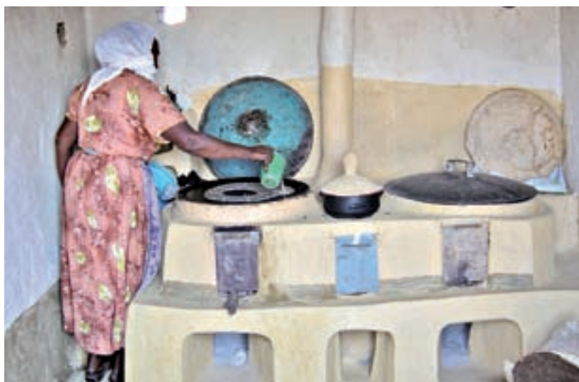
The energy-saving stove is designed to allow free flow of air through a cylindrical fire-holder, whose sides are built with curved ceramic hollow bricks insulated with ash or sand to minimize heat loss. The valve door and chimney minimize smoke emission into the kitchen. © LWF/DWS Eritrea/A. Fisseha
